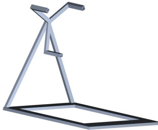
Figure 3-2 Sun Simulator mounting structure
