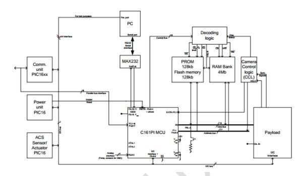
Simplified flowchart, introducing the idea of "one main processor":
