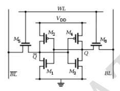
Generally static RAM memory is used. SRAM is a type of volatile memory with random access. It uses bistable latching circuitry to store each bit. Latches are storage cells. After setting one of two states it stores it until the power is disconnected. It doesn't require memory refreshing and is faster than DRAM so it is used as processors cache memory. Although it is more complicated and more expensive.
