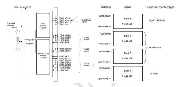
Connection of FSMC controller to the external SRAM memory:
