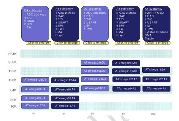
On-board computer requires reserve (OBC1) microcontroller with at least 3 I2C buses (control buses), 3 SPI buses (cameras and memory) and 1 UART interface (debugging). TWI that is two-wire interface (I2C). These requirements satisfy systems from the A1 series (column to the right). On the horizontal axis number of I/O ports were put. System from A1 series has 100 of them.
