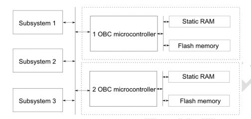
A disadvantage of this solution is that in two identical microcontrollers structure's degradation caused by ionizing radiation proceeds at similar rate. So when one microcontroller malfunctions due to this, there is high probability that the second one will be damaged in similar degree. Another problem is the space occupied on the board. Solution to this problem may be in the next subsection.
