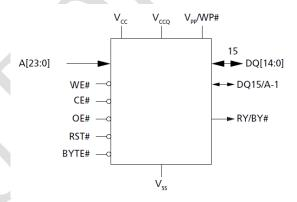
NOR Flash memory doesn't have such outputs such as UB and LB. Other outputs have the same functions as in SRAM memory. Additional memory outputs are, e.g.  $\overline{RST}$  reset system,  $\overline{RY}/\overline{BY}$  occupied memory information and  $\overline{BYTE}$  for 8 or 16-bit mode.
