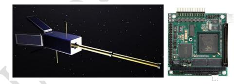
Main QuakeSat's computer was based on x86 processor which worked with 66MHz clock rate (Prometheus PC-104 ZFx86). At first its clock rate was 100MHz but it was lowed to 66MHz to reduce the amount of emitted heat. 32MB of RAM together with 192MB flash disk were installed. Everything was working under Red Hat 9 Linux operating system. Microcontroller PIC16F628-20P functioned as a hardware watchdog.
