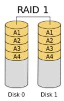
In order to boost the reliability two identical memory blocks can be used for settings data saving. Both blocks would have the same data, just like in RAID 1 hard disks array.
