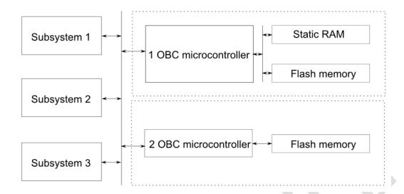
On the scheme above one can find the main microcontroller (number 1) and the secondary (redundant) microcontroller (number 2). No 1 takes care of processing images and sending images between cameras and OBC
