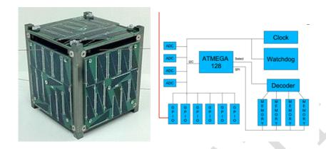
It was running on ATMega128 microcontroller with RTOS operating system. Data were stored on Flash memory with SPI interface.
