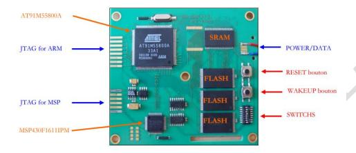
Space available on PCB board was utilized suboptimally. Two JTAG edge connectors take too much space. Tantalum capacitors aren't optimal choice for using in places which require high reliability.
