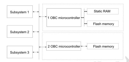
This diagram presents the idea of connecting two different microcontrollers. In this section it will be extended with memory blocks.
