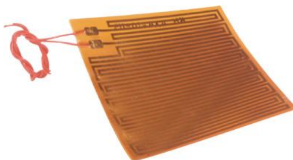
Figure 6-2 Kapton heater used to imitate heat source and dissipation
