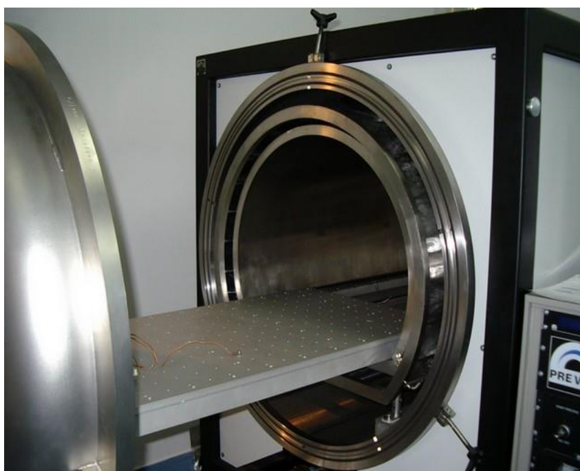
Figure 6-1 An example of a thermal vacuum chamber in CBK PAN
